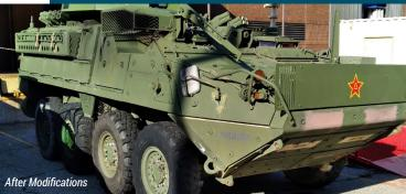
CALIBRE made bolt-on modifications to this Stryker vehicle to make it appear as a Chinese amphibious armored vehicle.
